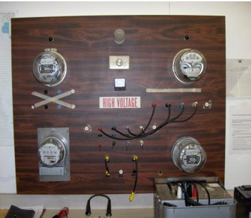
Electric Meter Test Board
