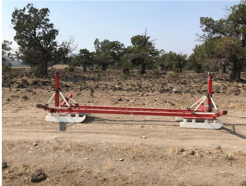
Figure 3 The tTEM transmitter sled setup.
