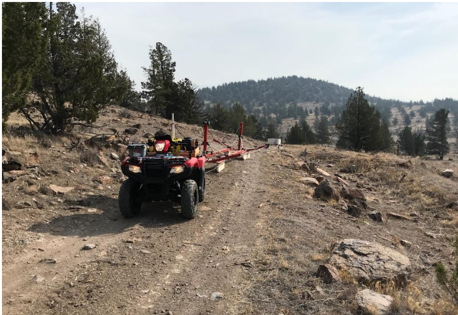
Figure 1 The tTEM system in operation at the site.
