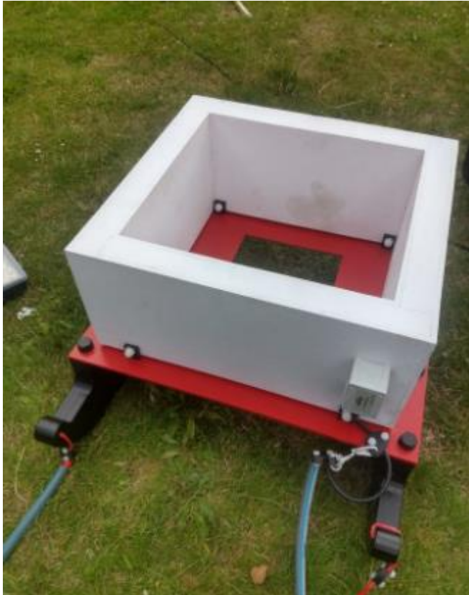
Figure A1- 5 The TEM Receiver coil is suspended to reduce motion induced noise.
