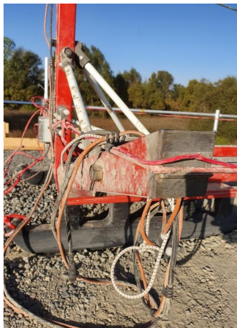
Figure A2- 2 Close-up photo showing the transmitter frame mounted on the sled
