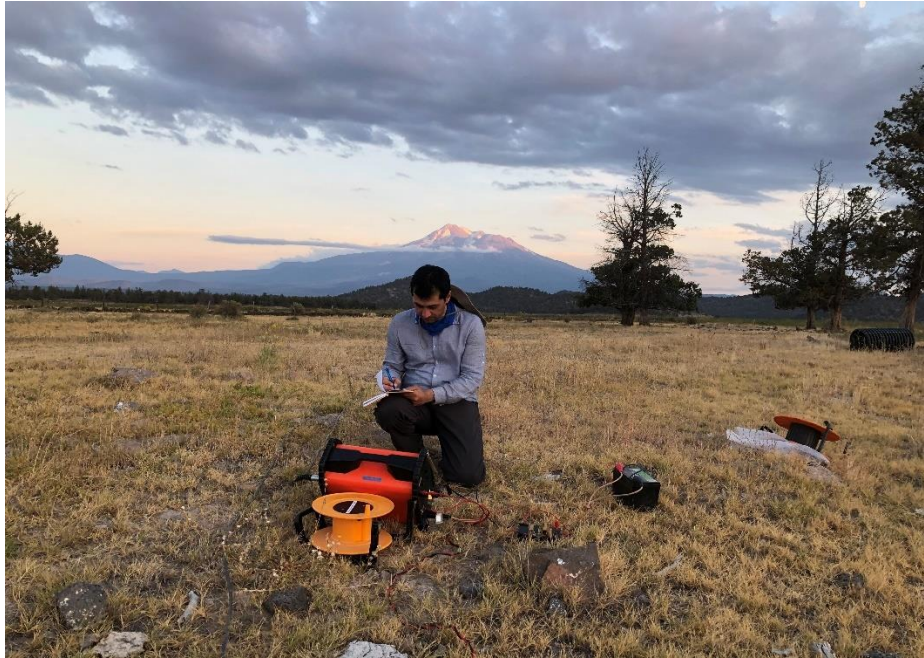
Figure 2 The WalkTEM system in operation at the site.
